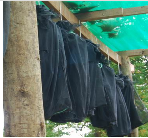
Figure 4: Insect-rearing 'sleeve cages' used for rearing wood-boring beetles out of pre-exposed timber baits.
